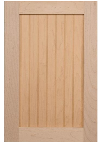
STYLE: SQUARE RAIL & STILE PROFILE: SHAKER PANEL PROFILE: BEADED FLAT PANEL OUTSIDE EDGE: EASEOVER WOOD SPECIES: PAINT GRADE MAPLE
