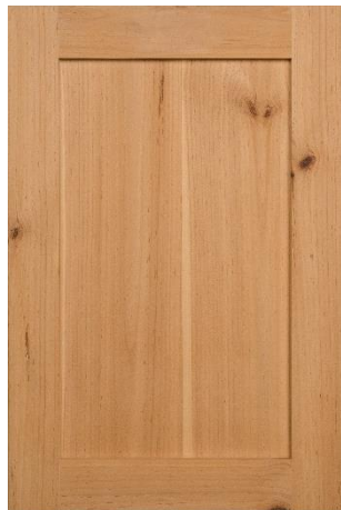
STYLE: SQUARE RAIL & STILE PROFILE: SHAKER PANEL PROFILE: REVERSED RECESSED OUTSIDE EDGE: ¼" with ROUND STEP WOOD SPECIES: KNOTTY PINE
